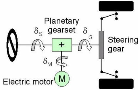
Figure 1: Schematic view of AFS system. The electric motor superimposes an angle  $\delta_M$  to the hand steering wheel angle  $\delta_S$ . The result is the steering gear's pinion angle  $\delta_G$ .
