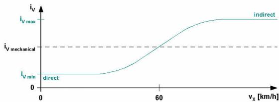
Figure 10: Example for velocity dependent ratio  $i_V(v_X, \cdot)$ .
