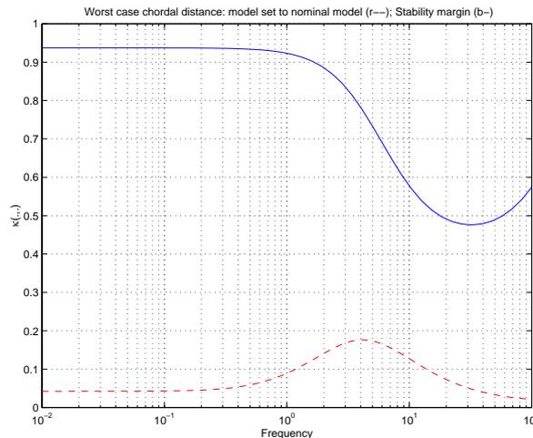
Figure 13: Pointwise worst case chordal distance from nominal model to model set (dashed red) and generalised stability margin  $\kappa(P_{nom}^{-1}, K_{\infty})$  (solid blue).
