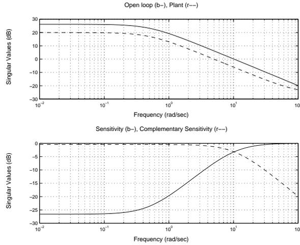
Figure 11: Singular values of plant and open loop (upper plot) and sensitivity function and complementary sensitivity function for the control system made up with controller and nominal model  $[K_\infty, P(\theta_{nom})]$ .
