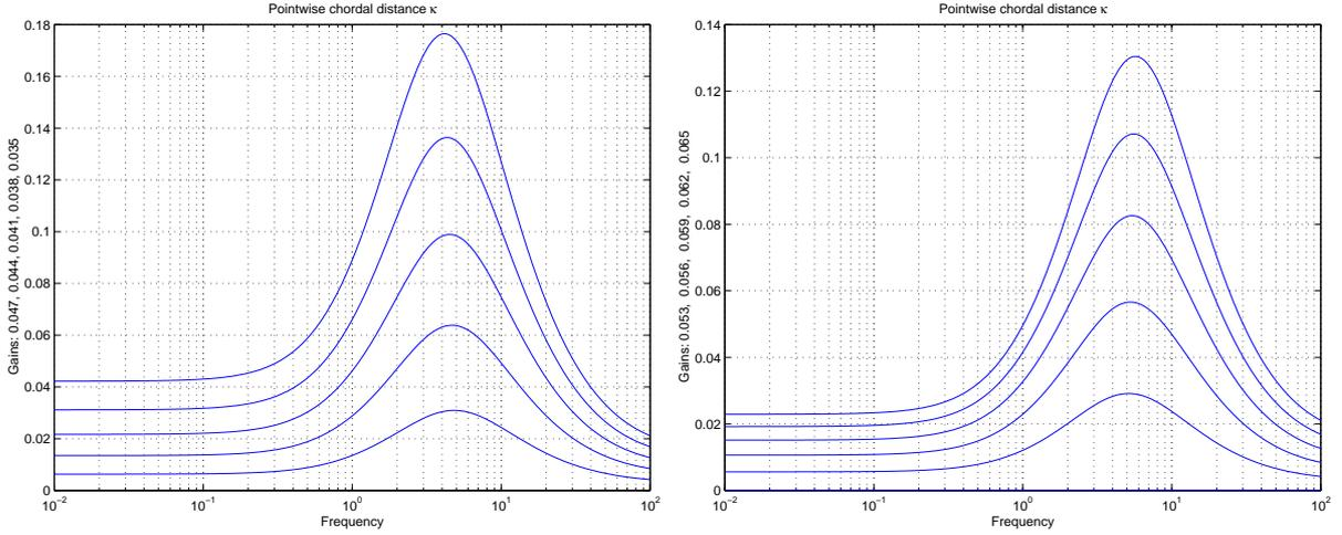
Figure 8: Pointwise chordal distance of certain members of the model set  $P(\theta_i)$  to the nominal model  $P(\theta_{nom})$ : result for gains  $\theta_i$  that are smaller and larger (respectively) than the nominal gain  $\theta_{nom}$  (left and right respectively). The numerical values of the gains  $\theta_i$  are indicated along the  $y$ -axis.
