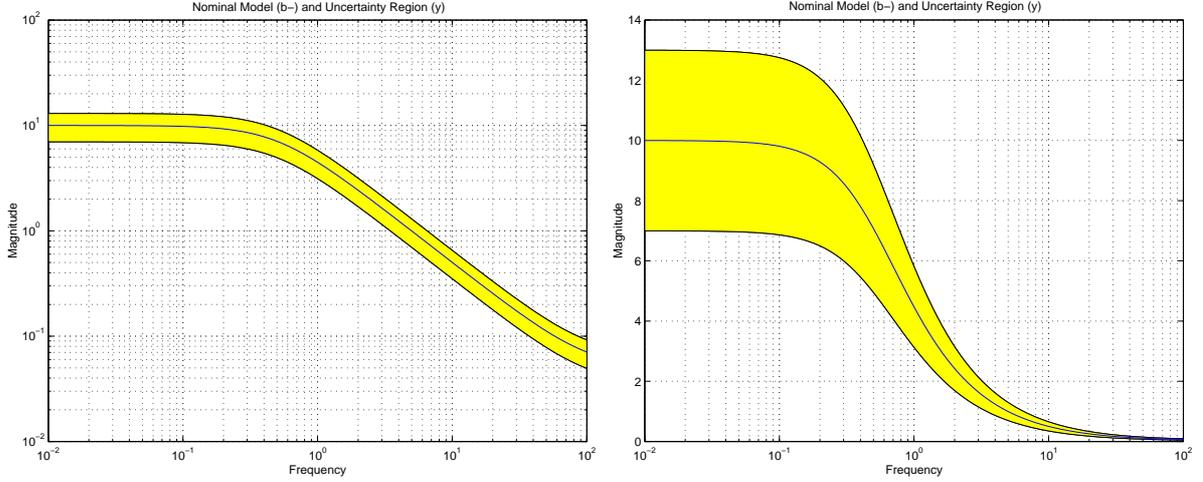
Figure 7: Nominal model (solid blue line) and its uncertainty region arising from the uncertain gain  $\theta \in \Theta$  in the frequency domain: logarithmic (left) and non-logarithmic (right).
