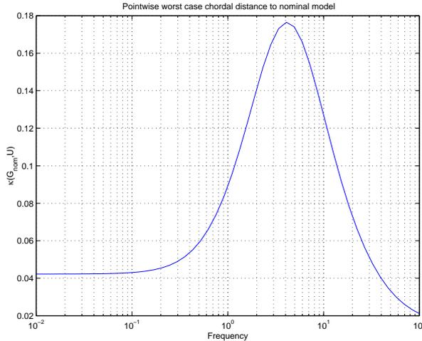
Figure 10: The pointwise worst case chordal distance from the nominal model  $P(\theta_{nom})$  to the model set  $P_{\Theta}$ , calculated using LMI optimisation.
