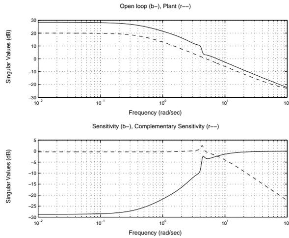
Figure 12: Singular values of plant and open loop (upper plot) and sensitivity function and complementary sensitivity function for the control system made up with controller and higher order model  $[K_\infty, P_7]$ .
