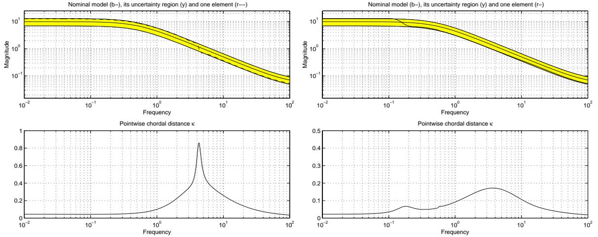
Figure 9: Upper plots: The systems  $P_7$  (left) and  $P_{1o}$  (right) and their location within the uncertainty set. Lower plots: Pointwise chordal distance from the nominal model  $P(\theta_{nom})$  to  $P_7$  (left) and  $P_{1o}$  (right).
